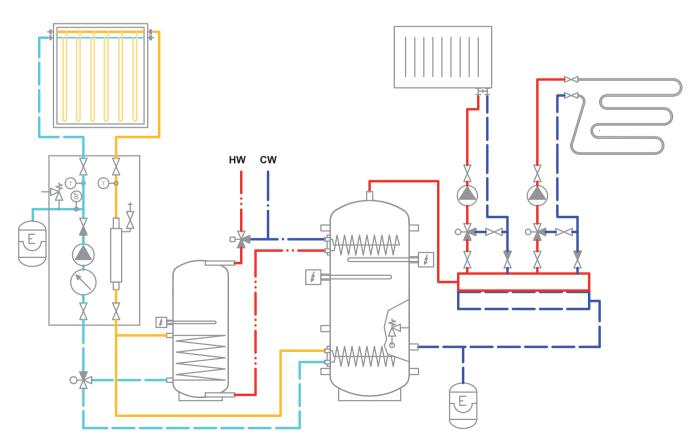
**Example II.**Solar collectors and combi gas boiler.
