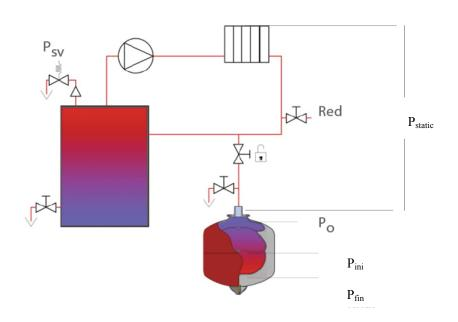
They are not suitable for use in open circuits with potable water or hydrocarbon fluids and those belonging to Group 1 in accordance with Directive 97/23 / EC. The content of glycol in water should not exceed 50%. Vessels are not suitable for placement outdoors.
